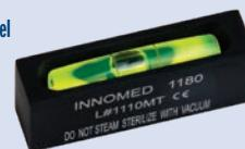
Helps to ensure the leg is in the same plane when initially putting the leg length caliper on and when reattaching the caliper.
