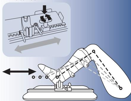
The Ratchet allows the Yoke Assembly to be moved in a precise gradual manner, the length of the Track. For faster adjustments, downward pressure on the Ratchet Handle releases the Yoke Assembly which then can be easily slid the length of the Track.
